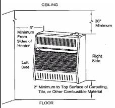
Figure 4 - Mounting Clearaances
